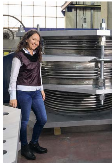
Bediha on site with an expansion joint.
