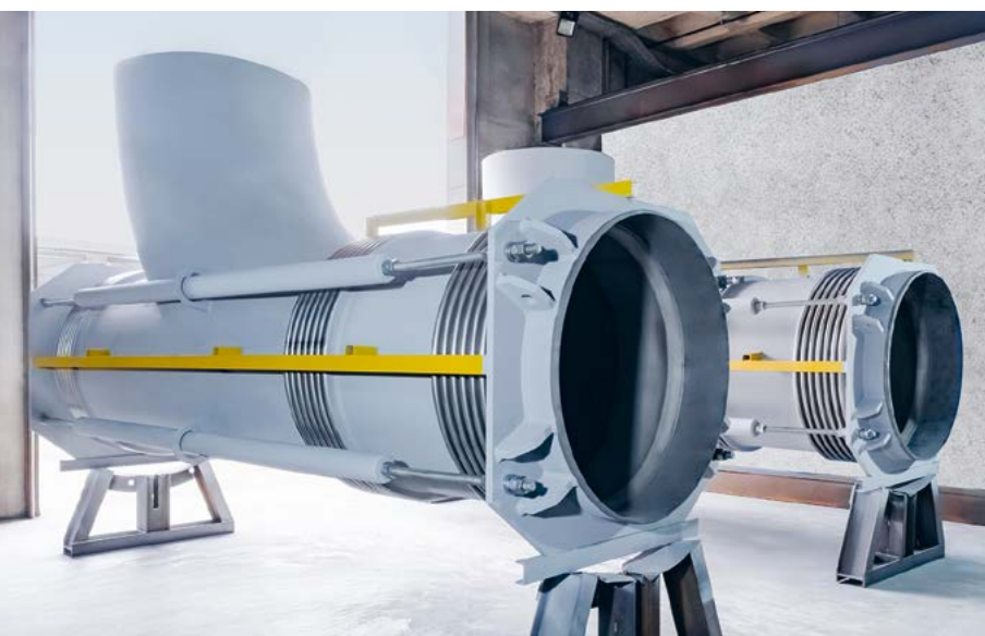
Custom expansion joints being prepared for Dradenau.
