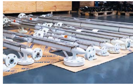
Hadro magnetic level gauges for a hydrogen plant.
