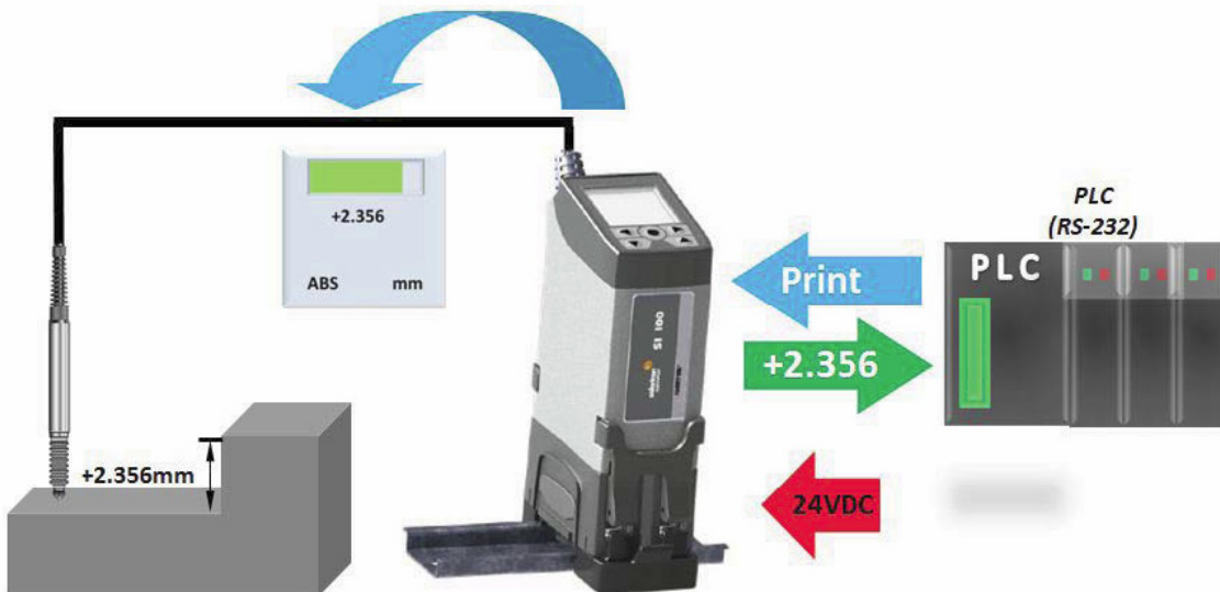
FROM MEASUREMENT SI100 to PLC via MODBUS
