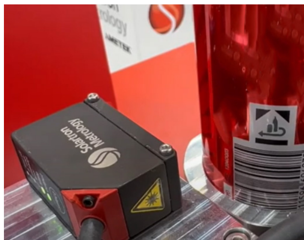
An LT2 sensor measuring the surface of a beverage can
