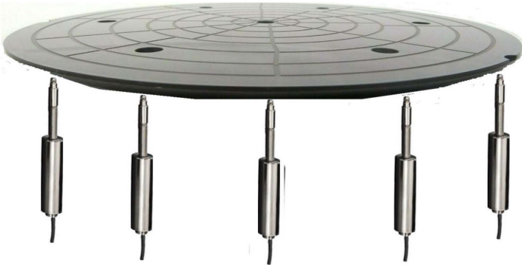
Component flatness being measured by G-Type Probes.
