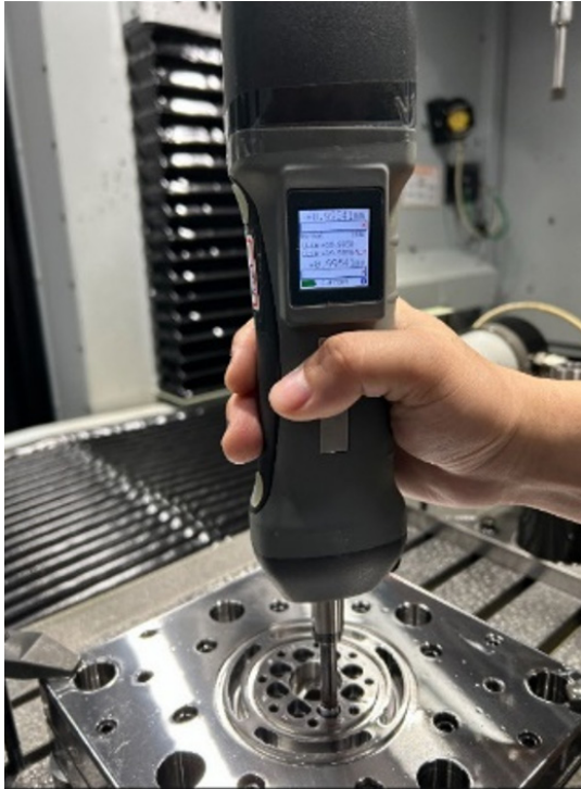
WiGauge™ Single Channel Wireless Hand Tool checking lens molds
