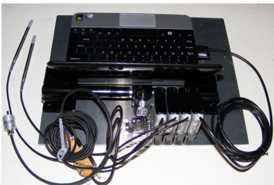
The Orbit® Digital Measurement Network connecting various products to record data
