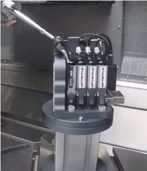
A 5-Axis machine using Digital Probes (DP) with a Wireless Interface Module (WIM) (Photo courtesy of Optifive in France, www.optifive.com )
