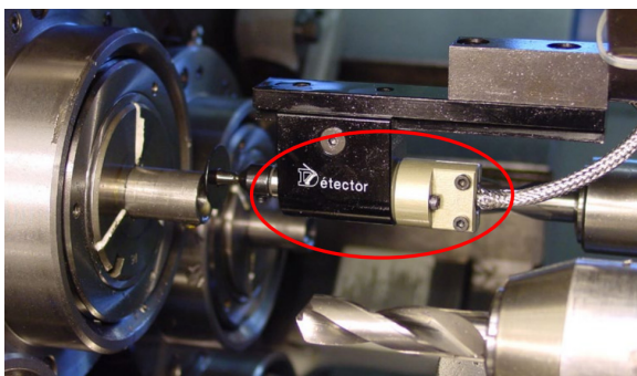
A Solartron probe is mounted into this Detector Length Measurer.
