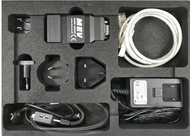
Figure 8.1 DMU41 Evaluation Kit
