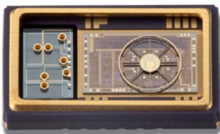
Figure 11.2 Combi-Sensor (Lid Removed)
