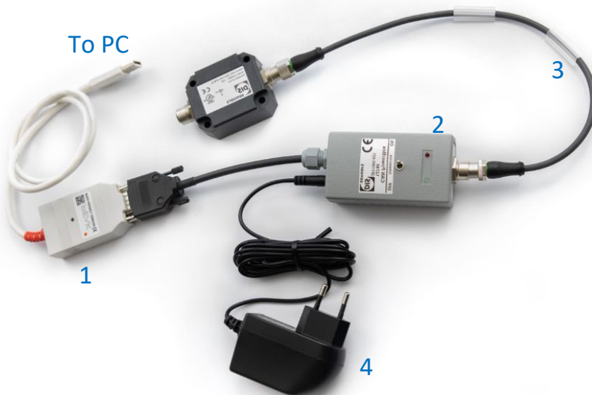
Figure 17 - Connection of DIS configurator set CAN
