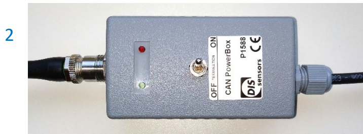
Figure 19 - CAN power box
