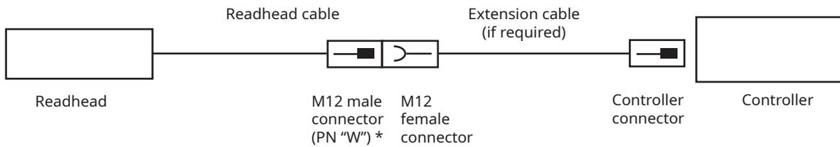
\* Input of the extension cable is M12 female overmould connector. When using an extension cable the LA12 readhead must be ordered with M12 (PN "W") connector.
