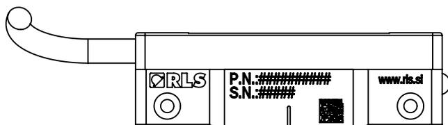
The engraving on the readhead contains a 20-digit part number, a 6-digit serial number and a QR code with a serial number.
