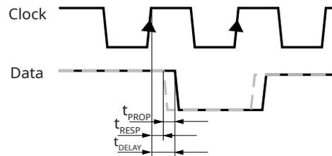
$$t_{DELAY} = t_{RESP} + t_{PROP} \times \text{cable length}$$
