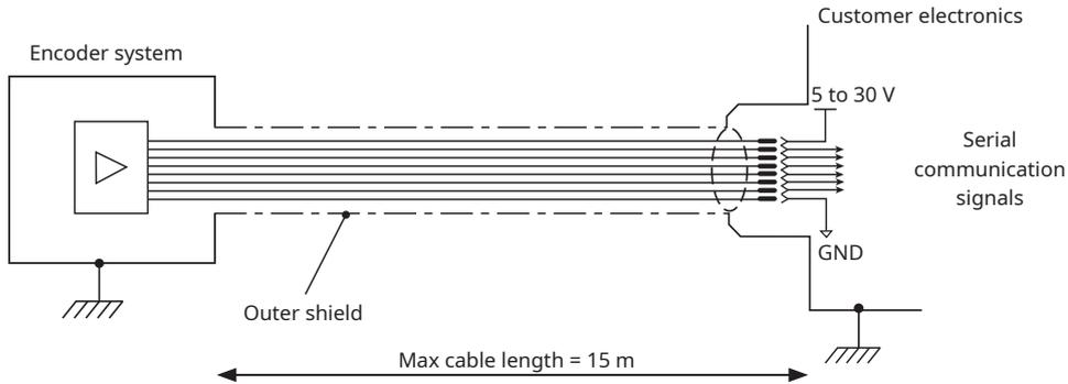
The encoder housing is galvanically connected to the connector housing. To achieve EMC compliance, the encoder system must be correctly integrated. In particular, attention to shielding arrangements is essential.
