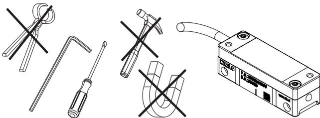
This encoder system is a high performance measuring instrument and should be handled with the same care as any other precision instrument. The use of industrial tools during installation or contact with strong magnets, such as a magnetic base, is not recommended as this risks damaging parts of the system which, as a result, may not function according to specifications.
