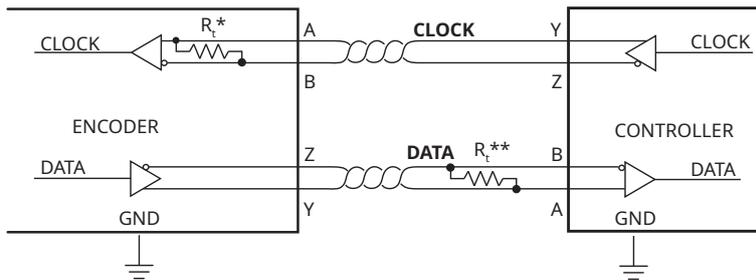
\* The CLOCK and DATA lines are 5 V RS422 compatible differential pairs. The termination resistor on the CLOCK line is integrated in the encoder.
