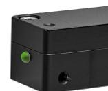
Slow flashing of LED indicates that the encoder is receiving power, but communication between the encoder and the controller has not yet been established. The error status has a higher priority than the warning status in the LED signaling. The signaling of LED may differ from the encoder status signaled by the controller. In case of error/warning the LED remains red/orange for at least 200 ms.
