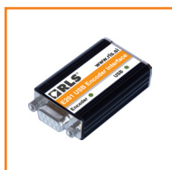
USB interface (ABZ incremental output) E201-9Q
